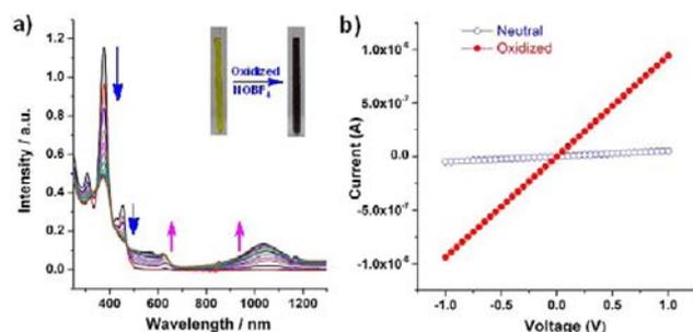
**Figure 8.** (a) UV titration upon adding  $\text{NOBF}_4$  solution to a solution of HTC<sub>Gemini</sub> in  $\text{CH}_2\text{Cl}_2$  (1 mM); (b)  $I$ - $V$  curve of a device fabricated from the nanofibers of HTC<sub>Gemini</sub> before and after oxidation with  $\text{NOBF}_4$  at  $25 \text{ }^\circ\text{C}$ .
